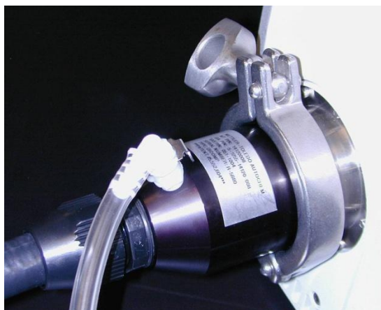
Main connection of fiber optic unit with purge line connected.
