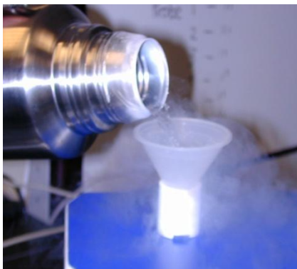
Filling the liquid nitrogen chamber
